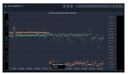
I/O BW of each OST over time before/after I/O subsystem problem indicated by vertical red colored bar (\* Focusing the slowest OST indicated by orange plots)
